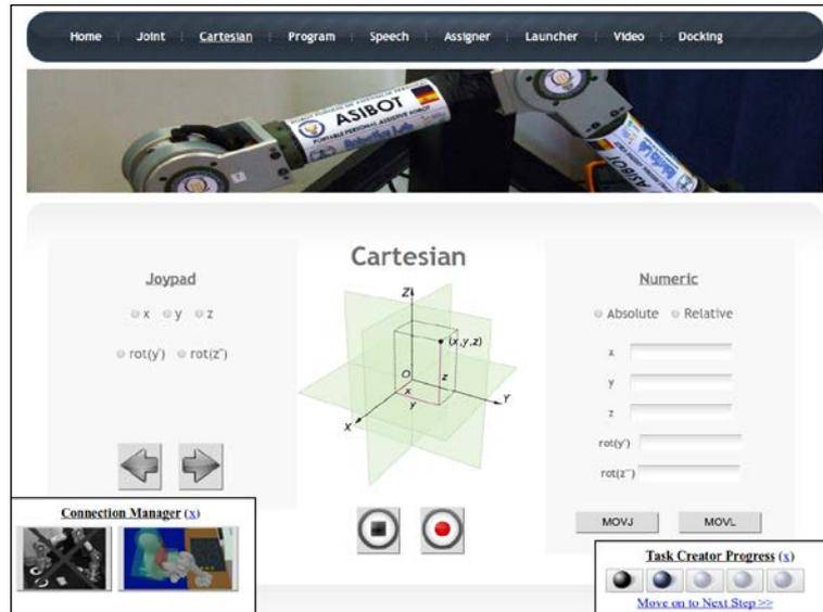
The capture button of either of these two tabs, namely the Joint space movement tab and the Cartesian Space movement tab, may additionally be used to capture points when the robot is moved by using the Wii Remote Plus controller interface. On the completion of this point capturing phase of the Task Creation process, the user is guided by the Wizard to the Program tab (see Fig. 6). Here, the user can create, edit, save and delete robot programs directly from within the Web Browsable interface.
