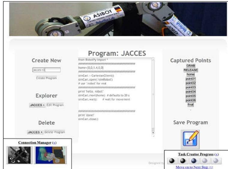
The Program tab additionally provides a set of buttons with the captured point names, situated on the top part of its right side panel. Clicking on this type of button inserts two lines of code into the central program text area:
