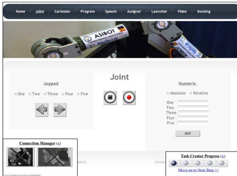
As previously mentioned, the user can establish connections with the real and the simulated robot using the persistent Connection Manager situated at the bottom left of the interface. Once the connections are established, the user can move the selected robots in the Joint space using the correspondent tab buttons.
