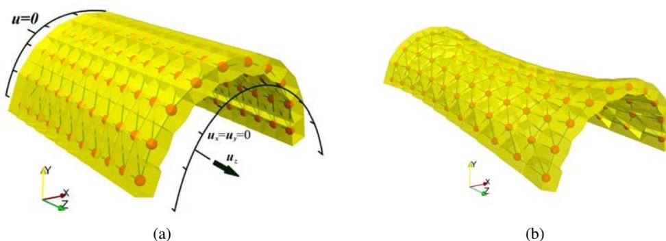
**Figure 3:** (a) Initial and (b) deformed shape for the curved monolayer test.
