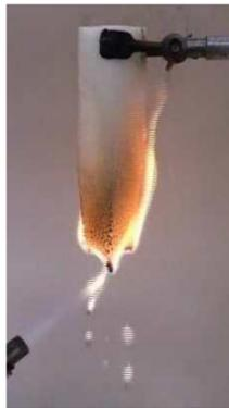
Figure 1: UL 94 test
