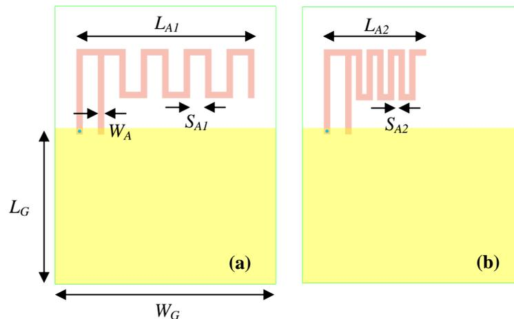
**Fig. 2.** Geometry of the (a) original and (b) redesigned meandered PIFA antenna.
