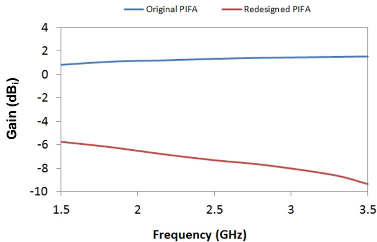
Fig. 5. Antenna gain for the (a) original and (b) redesigned meandered PIFA antenna.
