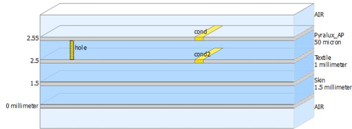
**Fig. 1.** Substrate definition including F-PCB, textile and skin effects.
