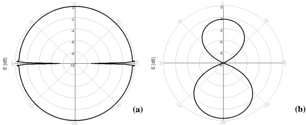
**Fig. 4.** Normalized radiation pattern for the maximum radiation level case at 2.45 GHz for the (a) original ( $\phi=141^\circ$ ) and (b) redesigned meandered PIFA antenna ( $\phi=177^\circ$ ).
