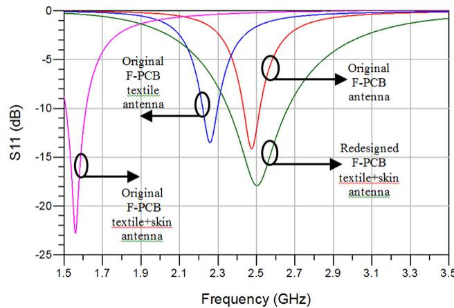
**Fig. 3.** Return loss of the original and redesigned PIFA antennas.
