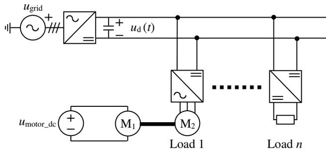
Figure 1. Structure of the LVDC grid
