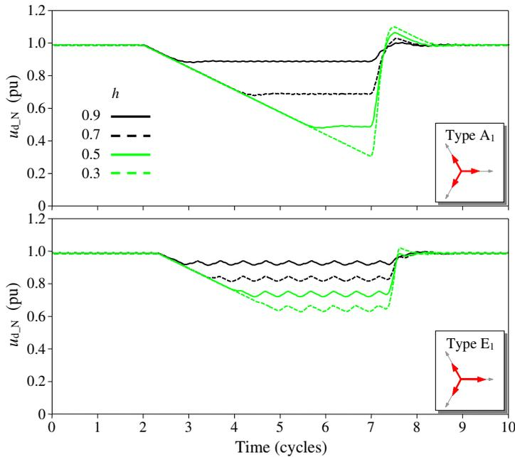
**Figure 4.** Analysis of dc voltage for different voltage sag depths.
