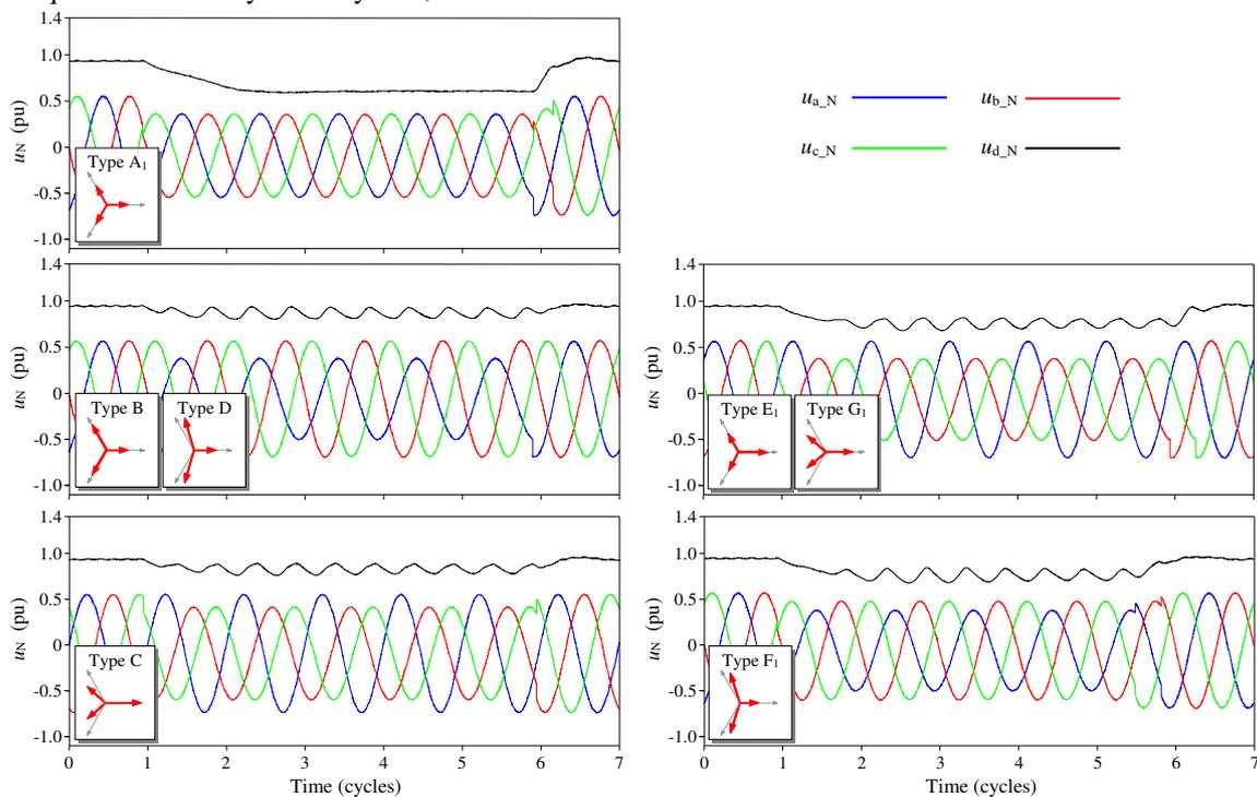
Figure 3. Measured effects of type A<sub>1</sub>, B, C, D, E<sub>1</sub>, F<sub>1</sub>, G<sub>1</sub> sags of characteristics  $\Delta t = 5T$ ,  $\psi = 80^\circ$ ,  $h = 0.7$ .
