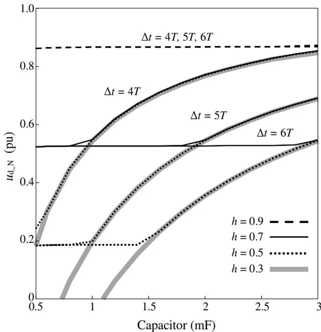
**Figure 5.** Analysis of dc voltage for different symmetrical voltage sag characteristics.
