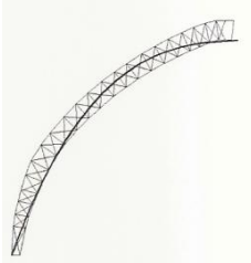
Fig. 23.-Funicular line of the third hypothesis.
