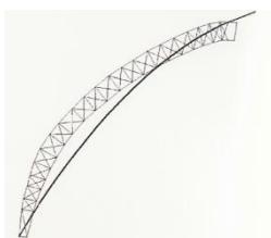
Fig. 22.-Funicular line of the central arc when the load of the roof has the value 2P/3 .
