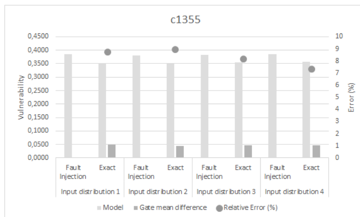
Fig. 6.18 Fault injection and Model comparison for c1355
