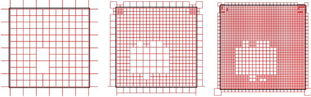
Figure 2: Problem 1. Example of the 2<sup>nd</sup>, 3<sup>rd</sup> and 4<sup>th</sup> meshes of the  $h$ -adaptive refinement process for  $Q_1$  elements.
