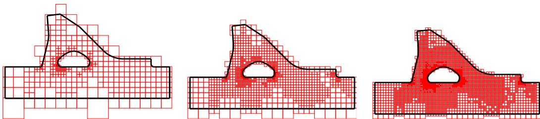
Figure 13: Problem 2. Example of the 2<sup>nd</sup>, 3<sup>rd</sup> and 4<sup>th</sup> meshes of the  $h$ -adaptive refinement process for  $Q_1$  elements.
