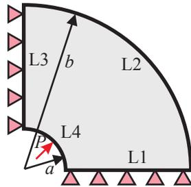
Figure 7: Problem 2. Thick-wall cylinder under internal pressure.
