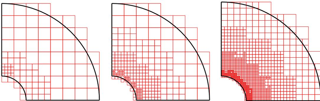
Figure 8: Problem 2. Example of the 2<sup>nd</sup>, 3<sup>rd</sup> and 4<sup>th</sup> meshes of the  $h$ -adaptive refinement process for  $Q_1$  elements.
