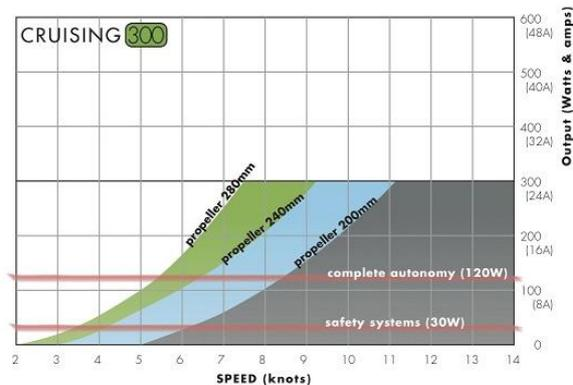
Fig. 9. Power - Speed curves of different hydrogenerator models [10]
