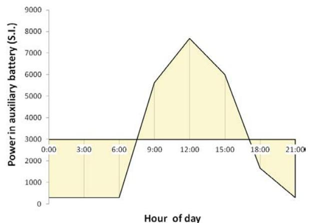
Fig. 11. Power in the auxiliary battery in an arbitrary spring-summer day
