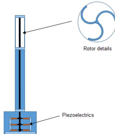
Figure 2 Configuration of turbine energy harvester device
