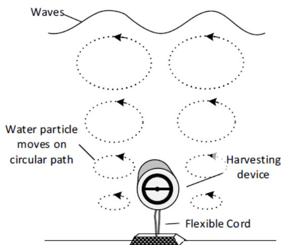
Figure 4 Configuration of motion energy conversion device
