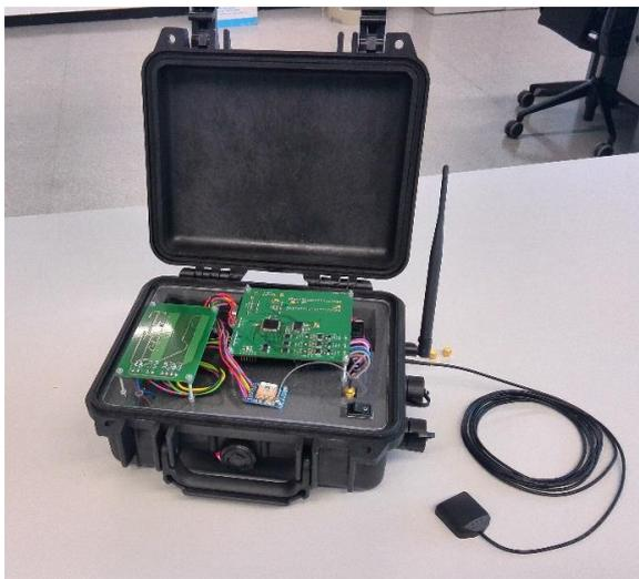
Figure 1 Volcanic seismic acquisition equipment
