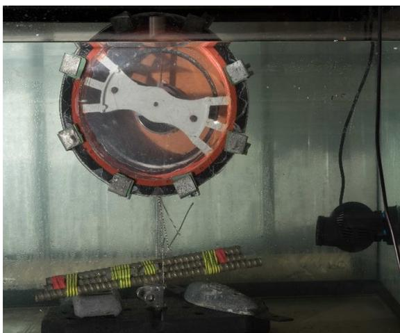
Figure 5 Sea motion electrical energy generator prototype
