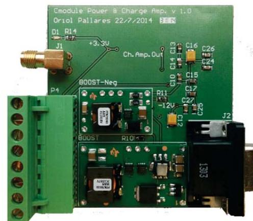
Figure 2. Power and charge amplifier front view.
