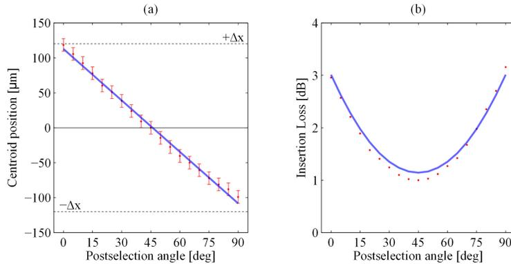
Fig. 4. (a) Measurement (dots) of the beam’s centroid position as a function of the postselection angle  $\beta$ . The solid line corresponds to a linear fit given by  $\langle x \rangle = -2.45\beta + 113 \mu\text{m}$  with correlation coefficient  $R = 0.998$ . (b) Measured insertion loss (dots) and theory (solid line) obtained from Eq. (4) with  $\Phi = 54^\circ$  as fitting parameter.
