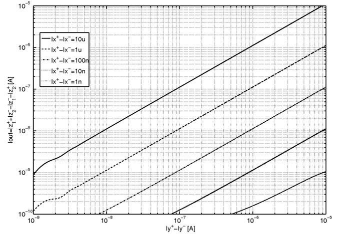
Figure 6. *Four-quadrant translinear multiplier log-scale DC response simulation at different tuning currents  $I_x = I_x^+ - I_x^-$ :  $10 \mu A$ ,  $1 \mu A$ ,  $100 nA$ ,  $10 nA$ ,  $1 nA$*
