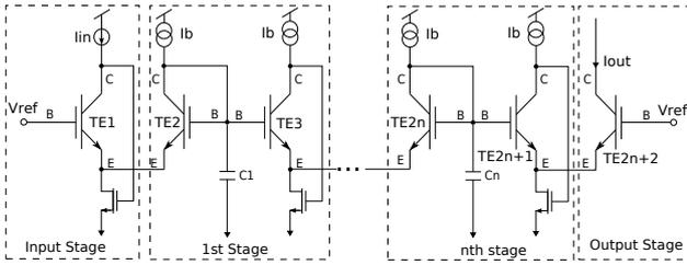
Figure 4. *nth-order low-pass filter schematic*
