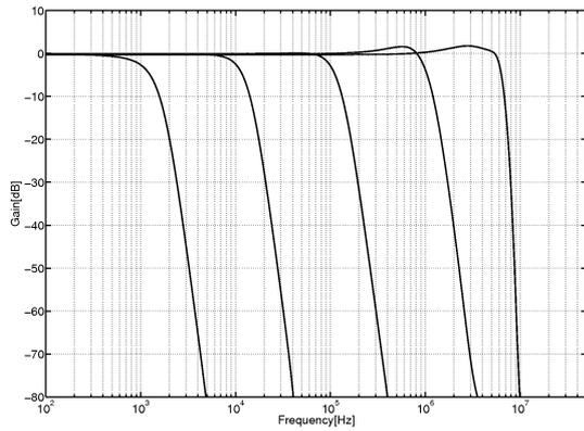
Figure 8. Fourth-order low-pass filter. Frequency Response at different tuning currents. From left to right tuning current  $I_b$  is: 1 nA, 10 nA, 100 nA, 1  $\mu$ A and 10  $\mu$ A, with a capacitance of 2.5 pF.
