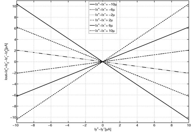
Figure 5. *Four-quadrant translinear multiplier DC response at different tuning currents  $I_x = I_x^+ - I_x^-$ :  $-10 \mu A$ ,  $-6 \mu A$ ,  $-2 \mu A$ ,  $2 \mu A$ ,  $6 \mu A$  and  $10 \mu A$*
