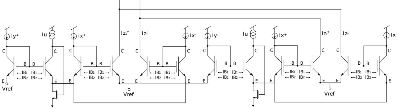
Figure 2. Four-quadrant multiplier schematic
