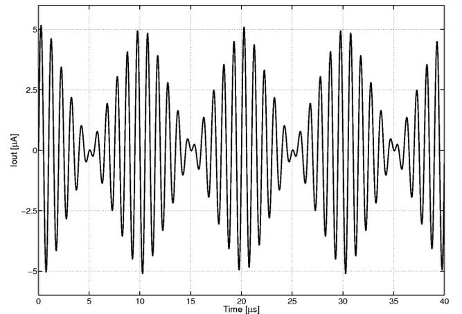
Figure 7. *Transient response of the four-quadrant translinear multiplier*
