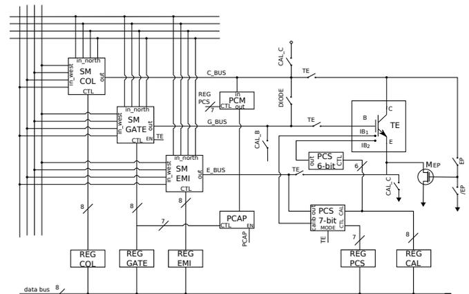
Figure 1. Block diagram of the Reconfigurable Translinear Cell (RTC) [2]
