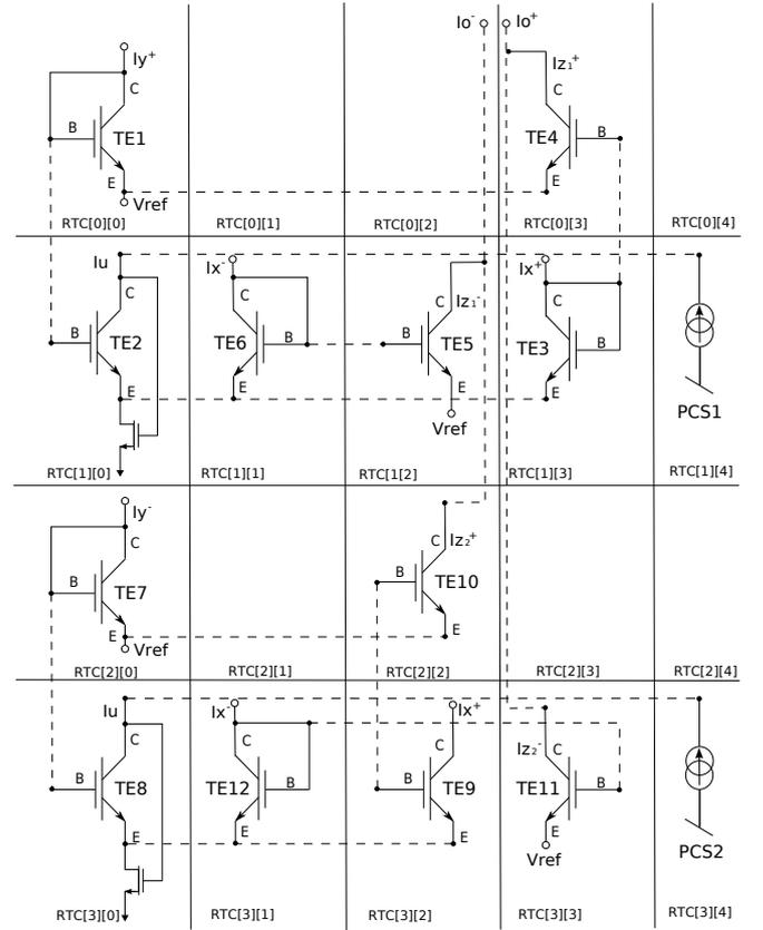
Figure 3. Four-quadrant multiplier mapping
