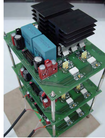
Fig. 5: Three-level three-leg dc-ac converter. (a) Topology. (b) Prototype using 150 V MOSFETs as devices S_{xi} .
