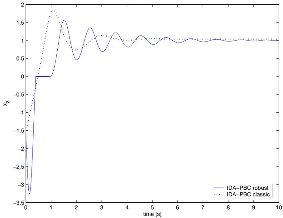
Figure 3: Comparison between the *robust method* and the *classic* IDA-PBC, behaviour of  $x_2$ .
