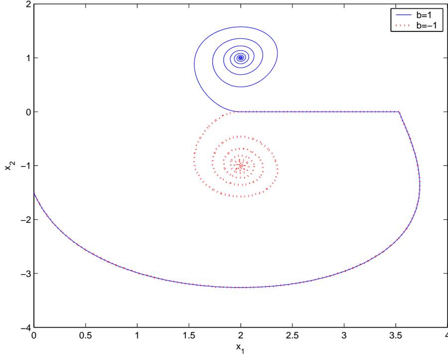
Figure 5: Phase portrait of  $x$  for two different  $b$  values.  $b = 1$  with a continuous line and  $b = -1$  with a dotted line.
