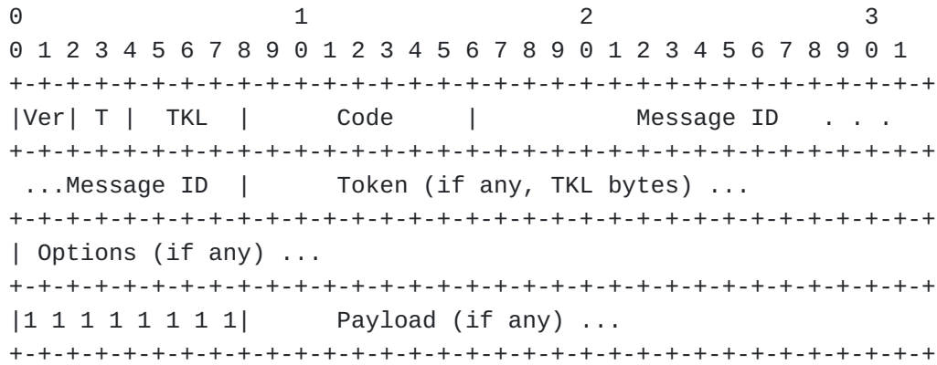
Figure 3: CoAP Message Format as defined in RFC 7252
