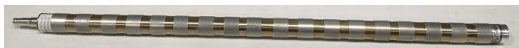
Fig. 1. 60-cm length and 1-inch diameter ^3\text{He} -filled proportional counter partially covered with cadmium to provide the detector with a flat efficiency.
