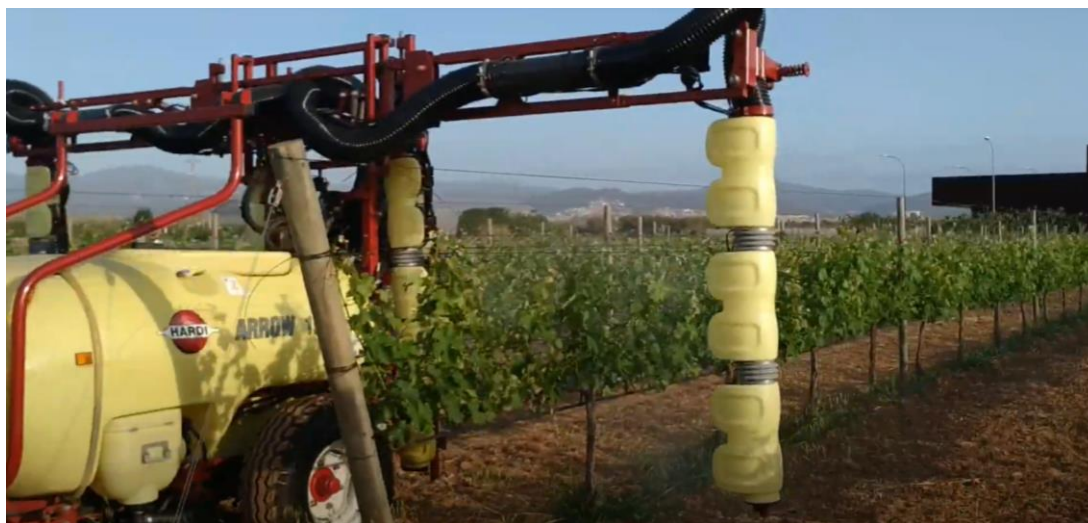
Fig. 2. Hardi Arrow Ilemo sprayer. Spray application of the Formulate 4 in field tests.
