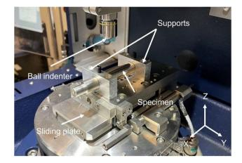
Fig. 2 Tribology setup for the new customized test
