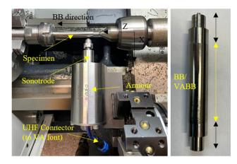
Fig. 1 Ball-burnishing tool and Ti6Al4V tribology sample
