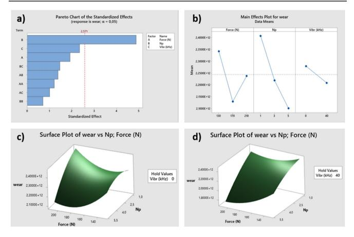
Fig. 8 a Pareto Chart being wear as the output. b ANOVA main effect plot being wear as the. c Surface plot for BB's sample wear. d Surface plot for VABB's samples wear
