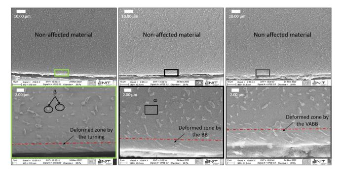
Fig. 4 Cross-section microstructures by columns: 1st column corresponding to machined surface, 2nd column corresponding to the 130–5-0 sample (BB), and 3rd column corresponding to the 130–5-40 sample (VABB)
