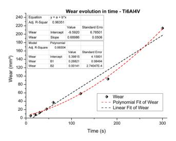
Fig. 9 Wear evolution along the time with sample 170–3-40
