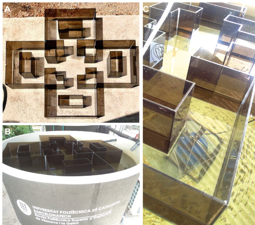
Fig. 1. Aquatic plus maze set-up. A: Shape of the aquatic plus maze. B: The maze in the tank. C: The underwater transducer placed 1 m below the maze on the tank floor is visible.
