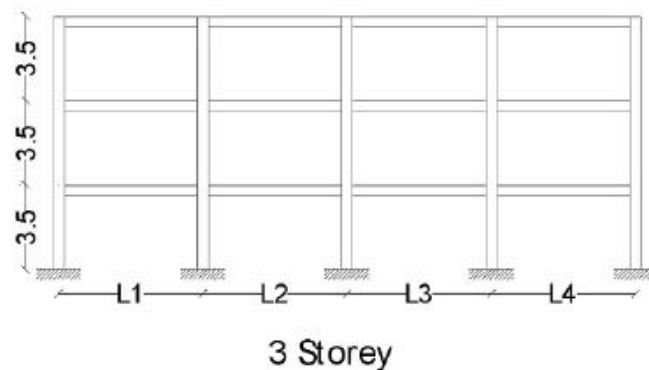
Figure 3.2 Frame 3 storey. Data source: (Lemma et al., 2022)
