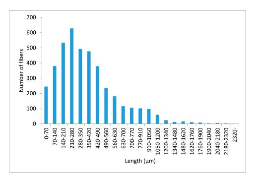
Figure 5. Fiber length distribution of the ONPF extracted from a 30% *w/w* composite.
