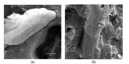
**Figure 2.** Micrographs of old newspaper fibers (ONPF) reinforced polypropylene (PP) composites, uncoupled (**a**) and coupled with a 6% w/w polypropylene functionalized with maleic anhydride (MAPP) (**b**).
