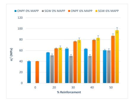
**Figure 4.** Comparison of the flexural strengths of coupled and uncoupled ONPF and SGW reinforced PP composites.
