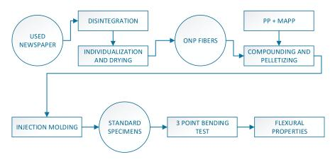
Figure 1. Flowchart of the research, from the raw materials to the experimental data.
