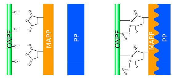
Figure 3. Schematic interactions between ONPF, PP and MAPP in the composite interphase.
