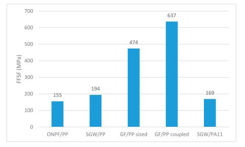
Figure 8. Fiber flexural strength factor of PP and PA11-based composites, reinforced with different fibers.
