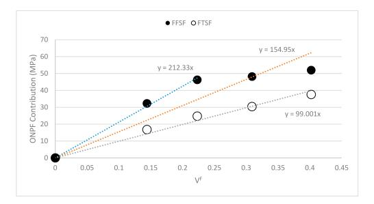
**Figure 7.** Fiber flexural strength factor and fiber tensile strength factor for the ONPF reinforced PP composites.
