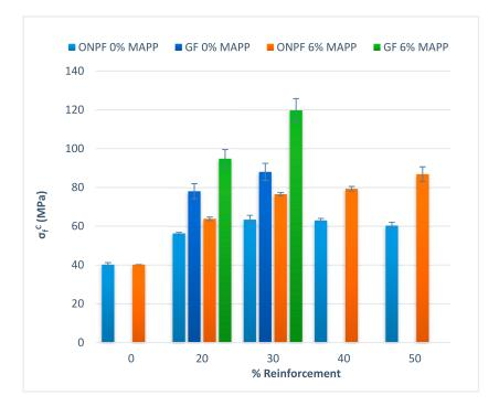
**Figure 6.** Comparison of the flexural strengths of coupled and uncoupled ONPF and GF reinforced PP composites.
