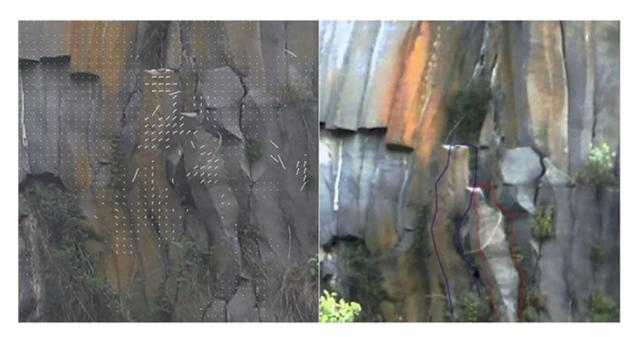
**Figure 8. Left**, movement vectors from camera 2. **Right**, in red and blue the original position of the columns.
