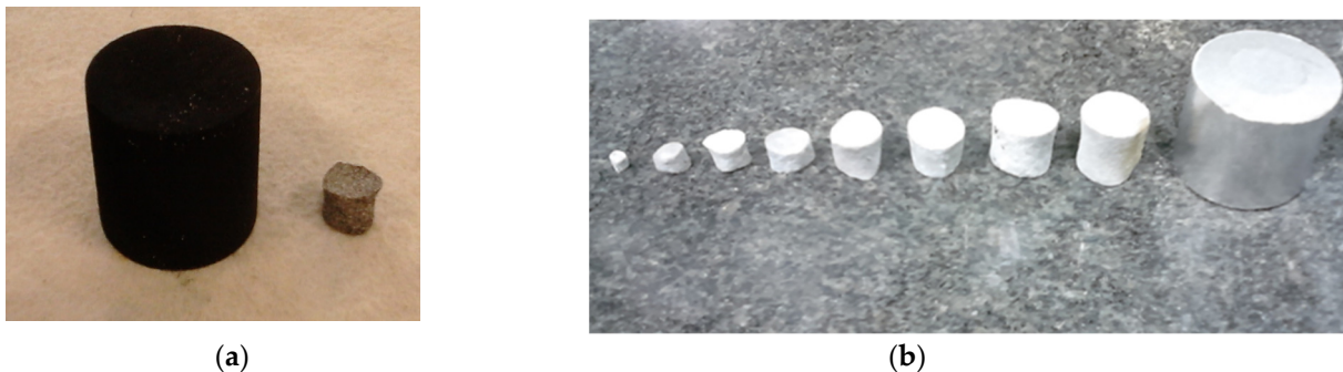
Figure 5. (a) Comparison between the residue of a totally solid specimen and that of pressed powder after approximately 2 h in a 6 M solution at 60 °C (0.015 mm/min surface [24]). (b) Evolution of a pressed-powder specimen fully submerged in a 6 M solution at 60 °C.
