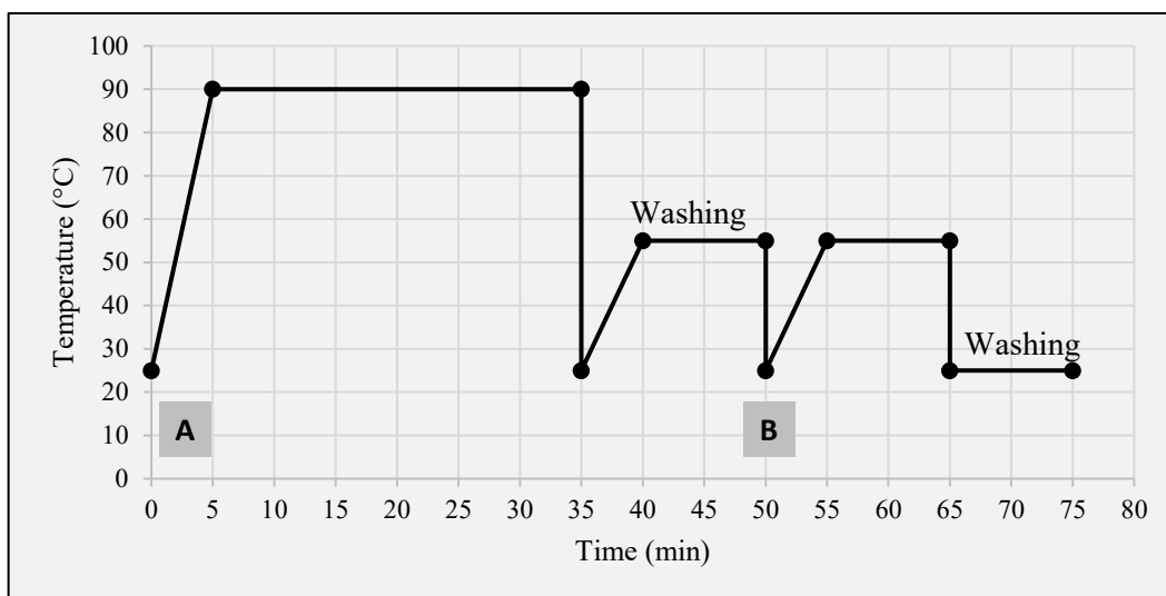
Suppl Figure 1 - Process scheme for enzymatic scouring of cotton knits. Solution A: BioPrep® 3000L (1.0 g L -1 ) and non-ionic surfactant (1.0 g L -1 ), in pH 8.5 buffer. Solution B: non-ionic surfactant (0.2 g L -1 ).
