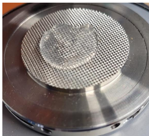
Figure 3.5. Hydrogel sample in the rheometer with the rough surface.
