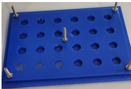
Figure 3.2. 3D-printed mold used to prepare alginate hydrogels.
