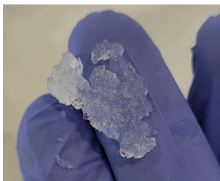
Figure 4.4. Picture showing the texture of an alginate hydrogel obtained using \text{CaSO}_4 as crosslinker and the Luer Lock syringe to mix before crosslinking.
