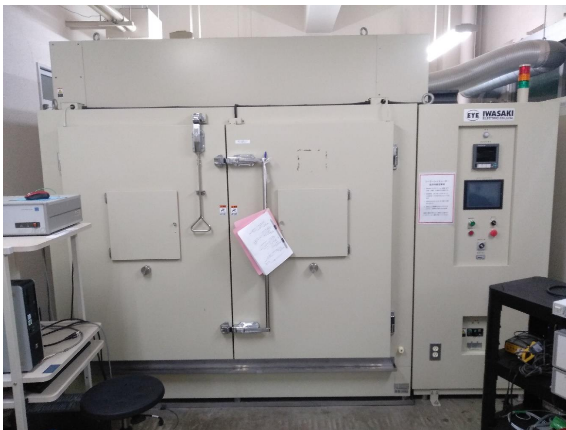
Image 13: Solar panel testing machine
