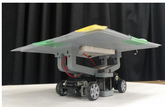
Image 18: Design of the support for the radio control car and photo of the current assembly
