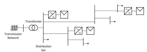
Fig. 8. Distributed photovoltaic generation (PVDG).
