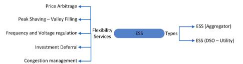
Fig. 6. Flexibility services of ESS.
