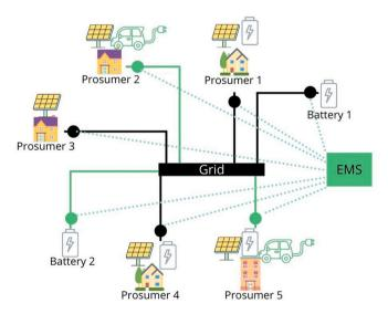
**Fig. 3.** VPP based on prosumers and microgrids with Energy Management System (EMS). Own preparation with pictures from Canva [68] from Note: Figure shows the activation of flexibility sources (green), e.g., prosumers, to respond a flexibility request.
