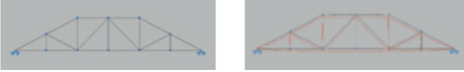
Figure 14. Deformation of a truss with triangular elements.
