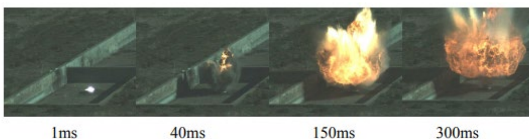
Figure 2. Reaction of pure TEA mixed with water (Liu et al., 2013)
