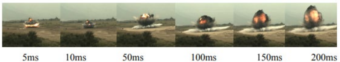
Figure 4. Explosive behavior of triethylaluminium in 50L vessel (Liu et al., 2013).
