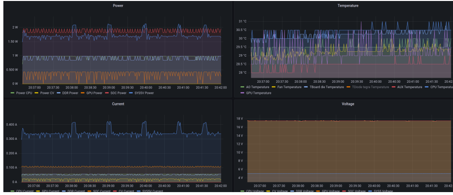
Fig. 5: NVIDIA Xavier Industrial power, voltage and thermals during the test in our custom Grafana-based control panel.
