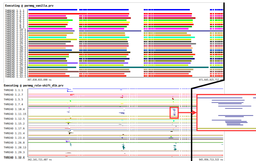
Figure 6.5: Paraver traces of three iterations using 32 MPI ranks. Top: vanilla version. Bottom: execution with role-shifting threads and DLB.
