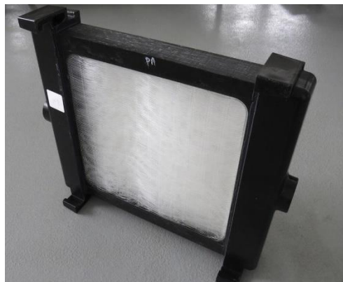
Figure 5. Hollow fiber automotive radiator prototype by Krásný et al. [11].
