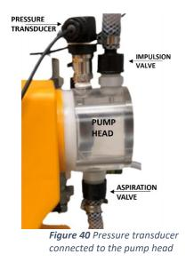
The pressure transducer acts as a variable resistor connected to a voltage source which gives a 4-20mA signal read by a DAQ System and the signal is then plotted (see **Figure 40** and **Figure 41**). The results obtained can be approximated by eq. (13)
