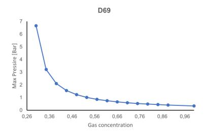
Figure 47 Maximum theoretycal pressure VS gas concentration for a D69 head.
