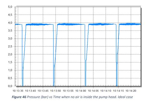
**Figure 46** shows the ideal case when the pump head is filled completely with liquid. The pressure is rapidly equalized to the backpressure and the constant region indicates that dosing process is taking place.
