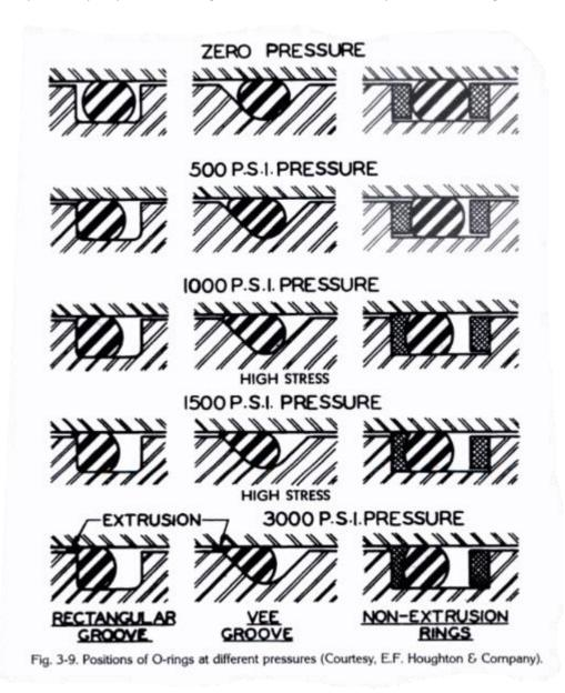
Figure 51 Positions of O-Rings at different pressures
