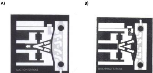
Figure 7: A) Suction process stroke; B) Discharge stroke process. From: ("Metering Pump Handbook - Robert E. McCabe, Philip G. Lanckton, William V. Dwyer - Google Llibres" n.d.)
