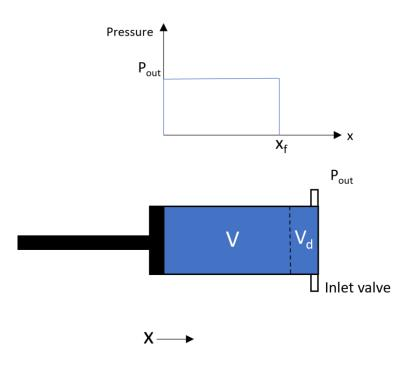
*Figure 31* Cylinder filled with liquid. Pressure equalizes instantly the out pressure
