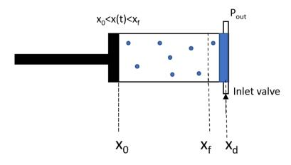
Figure 36 Piston pump with gas volume higher than V
