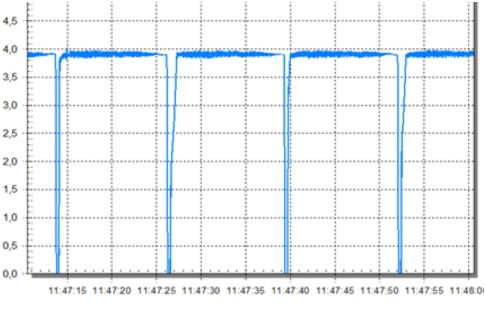
Figure 48 Pressure (bar) vs Time when a D69 head is filled with liquid
