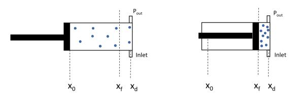
Figure 32 Initial and final position of the piston when the cylinder is completely filled with gas
