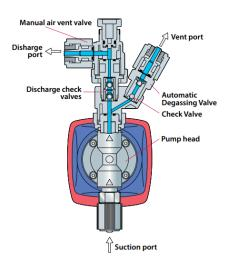
Figure 3: A secton view of an IWAKI degassing head
