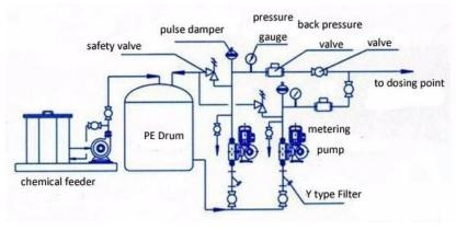
Figure 5: Typical metering pump installation. From: https://instrumentationtools.com/
