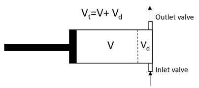
Figure 30 Piston cylinder model of a metering pump that is used to tackle this section
