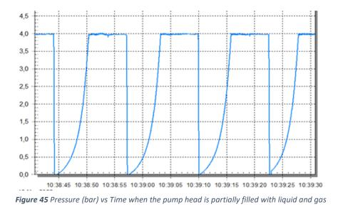
**Figure 45** Pressure (bar) vs Time when the pump head is partially filled with liquid and gasshows the mixed effects of having a pump head filled with gas and liquid corresponding to case 8.2.3.1. The process starts with an adiabatic curve due to the presence of gas until it reaches the backpressure, then the dosing process takes place and the curve turns constant. The experiments with the pressure transducer allow to corroborate the theoretical
