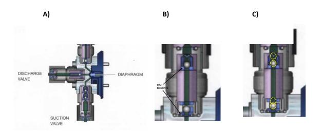
*Figure 2:* A) A secton view of a Prominent degassing head; B) Prominent degassing valve when suctioning; C) Prominent degassing valve when discharging
