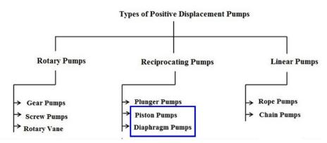
Figure 4: Classification of Positive Displacement Pumps
