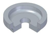
Figure 14 Lower O-Ring groove piece sectioned
