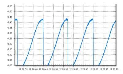
*Figure 43 Pressure (bar) vs Time in a D50 head filled with air.*
