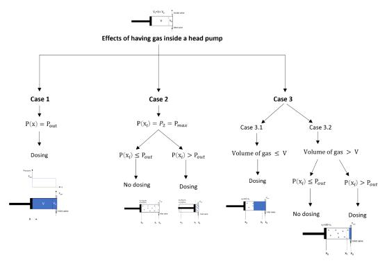
Figure 39 Scheme of the different cases when having air inside the pump head
