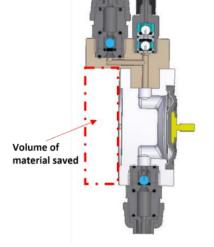
**Figure 29** Assembly of the pump, degassing head, purge valve, admission and impulsion valve. Proposal to reduce the environmental impact.
