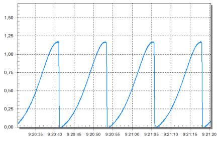
Figure 44 Pressure (bar) vs Time when half of the D50 pump head is filled with gas and half with liquid
