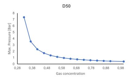
Figure 42 Maximum theoretycal pressure VS gas concentration for a D50 head.
