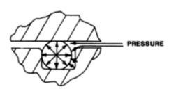
*Figure 18 Pressure distribution around the O-Ring. From: Metering pump Handbook*
