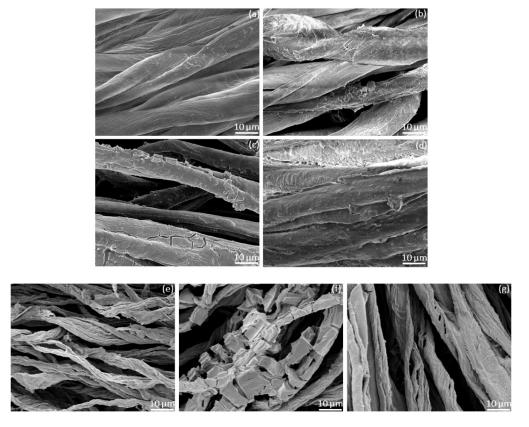
**Figure 4.** The SEM images of (**a**) pristine cotton; (**b**) C-Zr-MOF; (**c**) C-Zr-MOF/BPEI; (**d**) C-Zr-MOF/BPEI/VTES; (**e**) C-Zr-MOF residual chars; (**f**) C-Zr-MOF/BPEI residual chars; and (**g**) C-Zr-MOF/BPEI/VTES residual chars.
