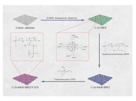
Figure 1. Graphical representation of the hybrid coating assembled onto cellulosic fibers.
