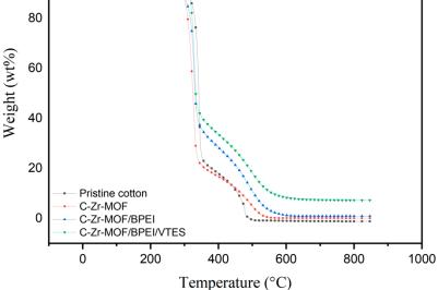
Figure 6. TGA curves of pristine cotton and treated samples.
