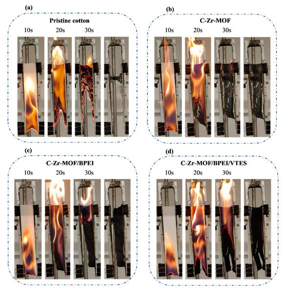
**Figure 3.** Digital photos of (**a**) pristine cotton; (**b**) C-Zr-MOF; (**c**) C-Zr-MOF/BPEI; and (**d**) C-Zr-MOF/BPEI/VTES in the vertical burning test after ignition.
