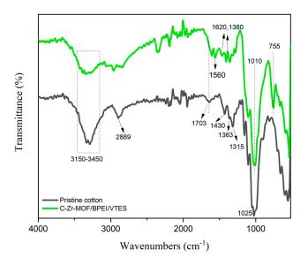
Figure 5. The FTIR spectra of the pristine cotton and C-Zr-MOF/BPEI/VTES sample.
