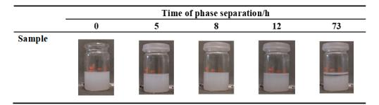
Figure 2. Digital photos of the Zr-MOF homogeneous dispersion at different times.
