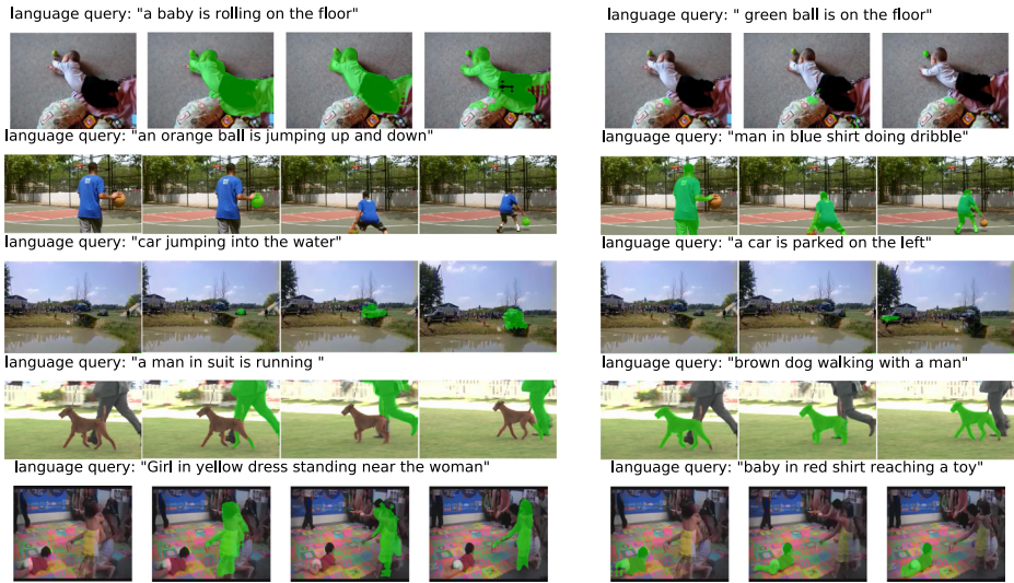
Fig. 6 Video sequences for A2D with expressions (language queries) and the results of our model. The first column shows a reference frame, the second to fourth columns depict the masks produced by our model when given the expression shown on top. Finally, the fifth to seventh columns show the results for the expression shown on top of these columns, which refers to another object of the video sequence
