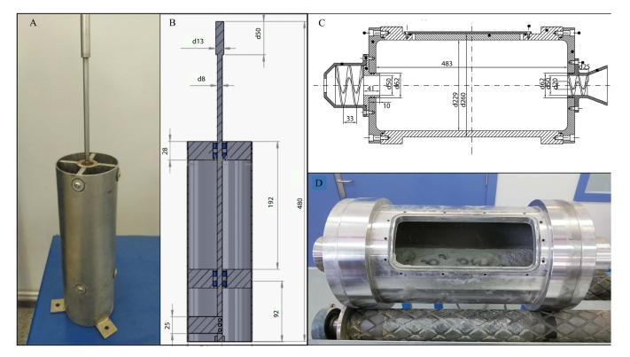
**Figure 2.** Attrition devices used in this study. (**A**) view of the attrition cell, (**B**) Plot of the attrition cell, (**C**) plot of the tumbling mill , (**D**) view of the tumbling mill.
