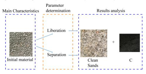
**Figure 1.** Work strategy scheme to evaluate liberation performance. In an initial stage we have raw material. After liberation and separation, the obtained material is a clean sand plus the removed volatile matter, which is mainly carbon.
