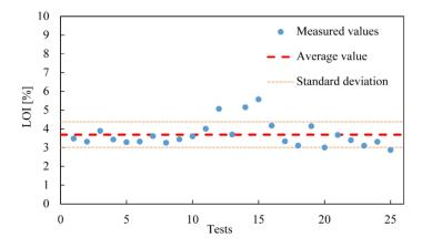
Figure 4. Results of the target waste material in terms of fixed carbon using the LOI technique.
