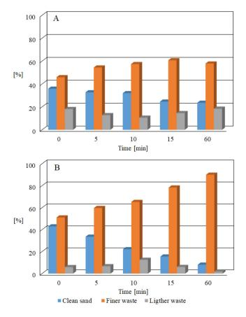
Figure 10. Contaminants distribution depending on process type. (A) By stirring (B), by light milling.
