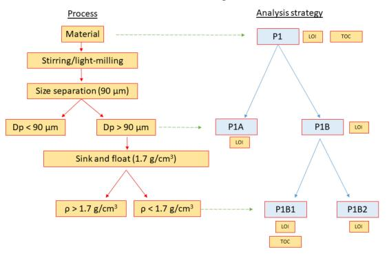
Figure 3. Scheme to obtain liberation of the volatile material contented in the sand, and analysis Scheme.
