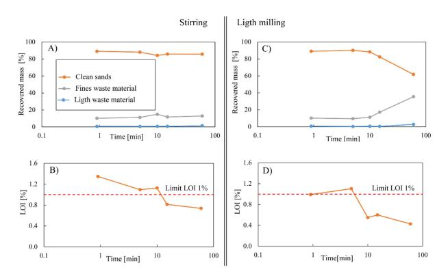
**Figure 8.** Comparative results of the liberation test. (A) Recovered mass using stirring, (B) LOI reduction using stirring, (C) recovered mass using light milling, (D) LOI reduction using light milling.
