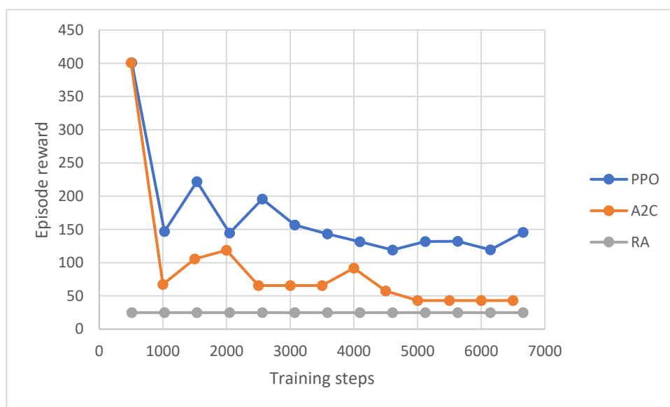
Figure 21. Evolution of episode reward during training using BC and 524 items when pretraining with the 5% of the set. PPO hyperparameters are the optimal: clip_range = 0,1 and clip_range_vf = 0,05.
