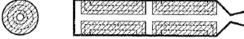
Figure 5.2: BATES grain regression. Source: [4].
