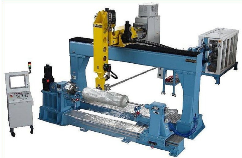
Figure 2.2: Filament winding machine for composite motor cases and pressure vessels manufacture. Source:
