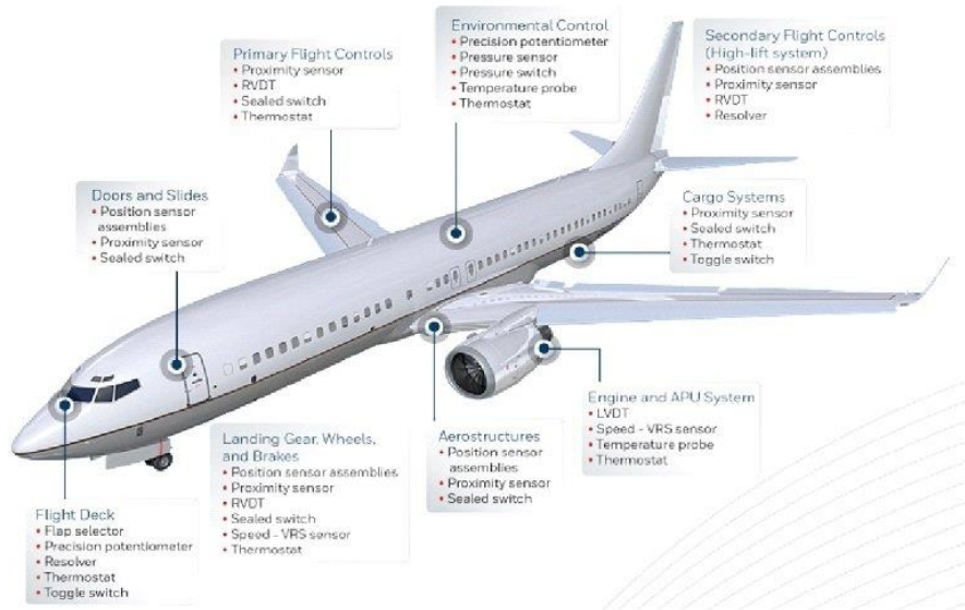
Figure 32. Aircraft system sensors II [151]
