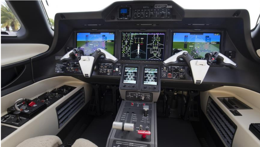
Figure 68. Embraer's Phenom 300E Prodigy Touch G3000 Integrated Flight Deck [184]
