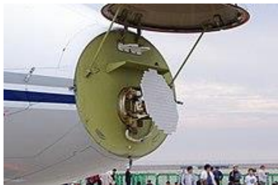
Figure 26. Weather Radar Antenna [146]
