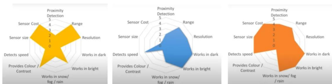
Figure 53. Characteristics of the most common DAA Technologies: Optical Cameras, LIDAR & RADAR, respectively [74]
