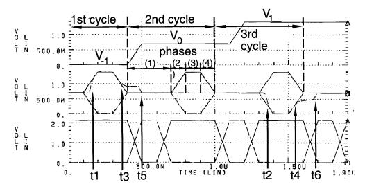
Fig. 2. Three different computational cycles of the STI for the three different inputs "-1," "0," and "1."
