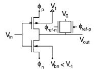
Fig. 6. Control of  $V_{tn}$  by using the body effect in order to have symmetrical logic levels.
