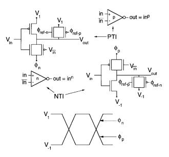
Fig. 3. Structures, symbols, and clocks of the NTI and PTI.
