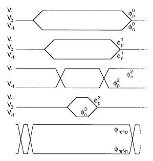
Fig. 5. Computing sequence of the power supplies for one phase of the pipeline.
