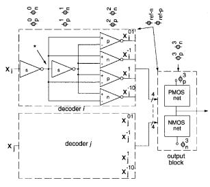
Fig. 4. Structure of a generic function in the QAT logic.
