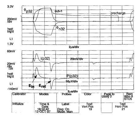
Fig. 9. Measurements of the multiplier.  $i_{p32}$  is the current from the clock  $\phi_{p32}$  and  $P_{p32}$  is the corresponding power.  $(E_{in} - E_{ret})$  is the energy dissipated in this switching.
