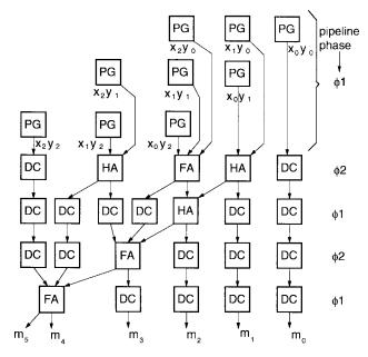
Fig. 8. Structure of a  $3 \times 3$  trits multiplier. PG are product generator cells, HA are half adders cells, FA are full adder cells, and DC are delay cells.
