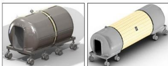
Figure 1 - The LaRC Expandable Lunar Habitat. Stowed and deployed
