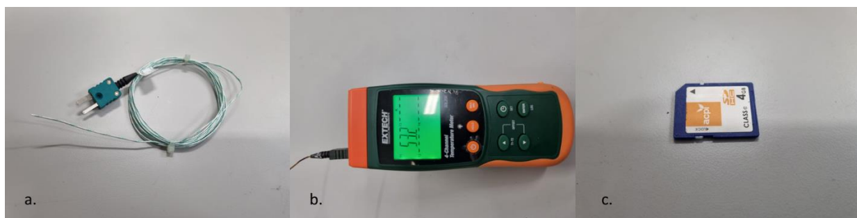
Figure 8. Figures of thermocouple (a), data logger (b), and memory card (c)
