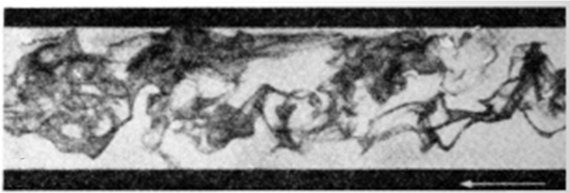
Figure 1.3: Reynolds experiment showing turbulent flow. [11]
