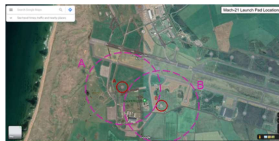
Figure 6: Landing Site Estimates - Launch Pad A and B locations in Red. In Pink dashed lines shows the effect of wind drift and shows landing region.
