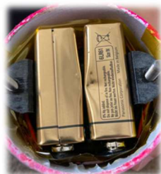
Figure 9: Post-flight damage to the batteries
