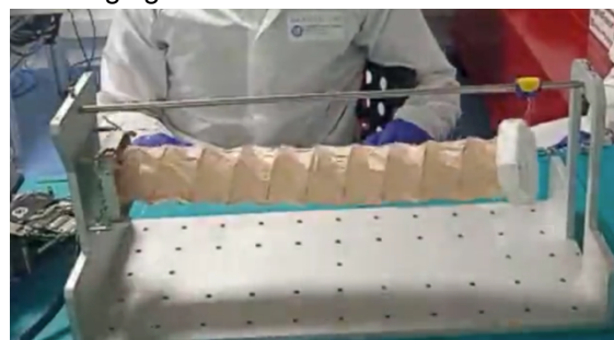
Figure 5. NADS subsystem ambient deployment
