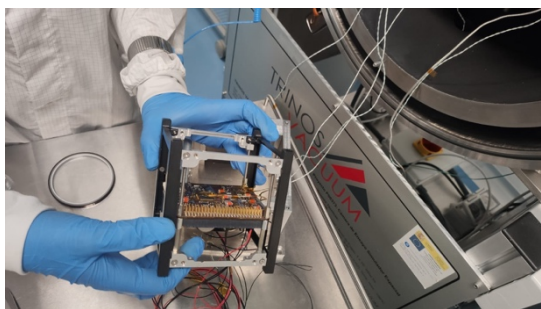
Figure 3. EPS subsystem preparation for TVAC testing
