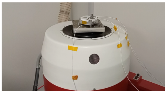
Figure 4. NADS subsystem vibrations test
