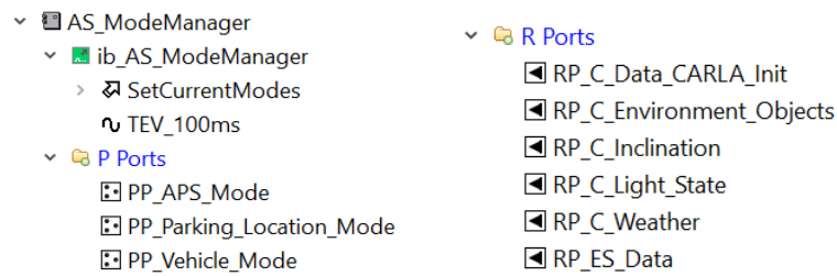
Figure 24. Ports and runnable configuration for the ADS Mode Manager.
