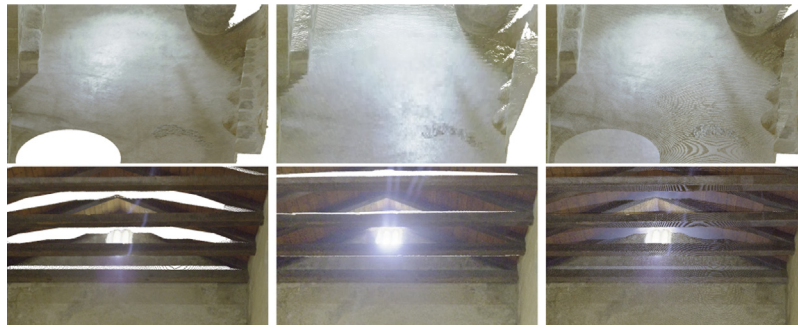
Fig. 18. Although our technique is able to correctly estimate gain factors in panoramas, view-dependent lighting effects such as specular reflections ( top ) and lens flares ( bottom ) will still produce artifacts when combining several scans into a single point cloud ( right ). Scan 20 is used on the left , scan 7 on top center and scan 19 in bottom center .
