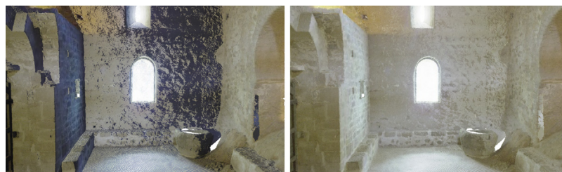
Fig. 14. Joint visualization of the point clouds acquired from scans 7 and 20 before (left) and after (right) applying our technique to the corresponding panoramas.
