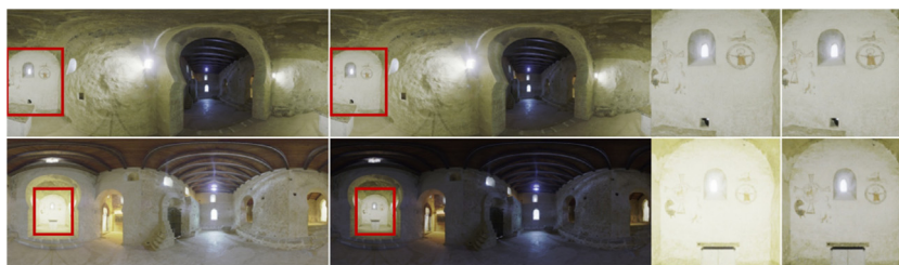
Fig. 16. White balance correction example (original panoramas and compensated ones) focusing on the central apse. Gain factors were optimized taking as reference scan 20 (outside the apse) but here we applied them taking as reference scan 04 (inside the apse), i.e. we applied gain factors \lambda_{q_i}^c / \lambda_{q_{04}}^c instead of \lambda_{q_i}^c . The white balance improvement can be seen by comparing the last column to that in Fig. 13.
