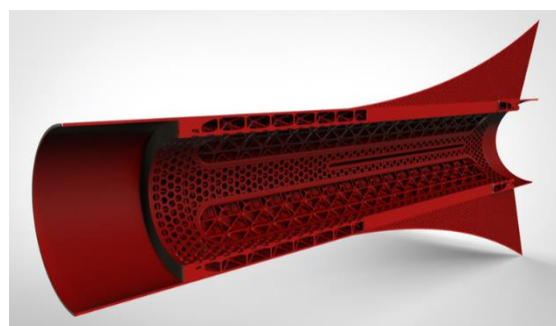
Figure 8. Generative design on the Ares III's motor section structure
