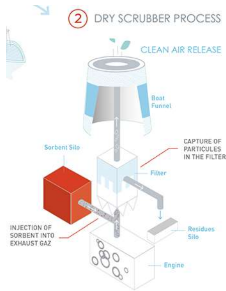
Figura 11. Scrubber sec – (font 11)
